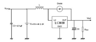
Hold-on voltage test circuit (I<sub>load</sub>=1mA)
