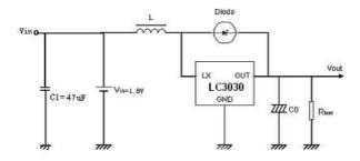
Start-up voltage test circuit (I<sub>load</sub>=1mA)
